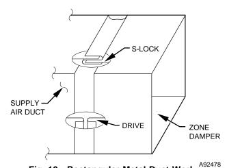
Fig. 10—Rectangular Metal Duct Work
